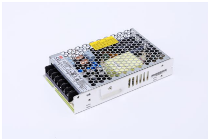
LRS-150 恒压 12V/24V/48V
