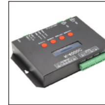
Programmable magic controller K-4000C DC5-24V DMX512 Signal
