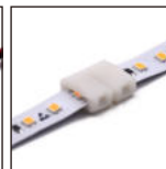
3PIN-8MM PCB to PCB
