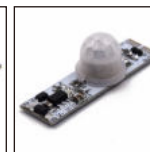
Human IR sensor sense personnel approaching >3m,DC12-24V
