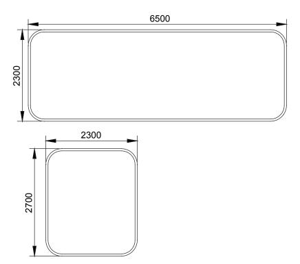
Input Voltage:AC180-240V Power:280W CCT:3000K Size:6500\*2300mm Corner: R=400mm
