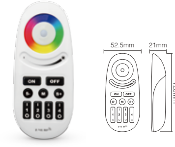
Model No.: FUT095 4-Zone RGBW Remote Control With Button RGB+W Color changing, brightness control Individed 4-zone group lighting separately, no bulb qty limited
